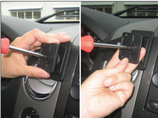
3. Start to thread the center screw into the base plate. When you connect with the nut pull the holder towards you to prevent the nut from spinning around. Continue to tighten the screw firmly. Then loosen the screw slightly for easier angling/rotation of the holder.
