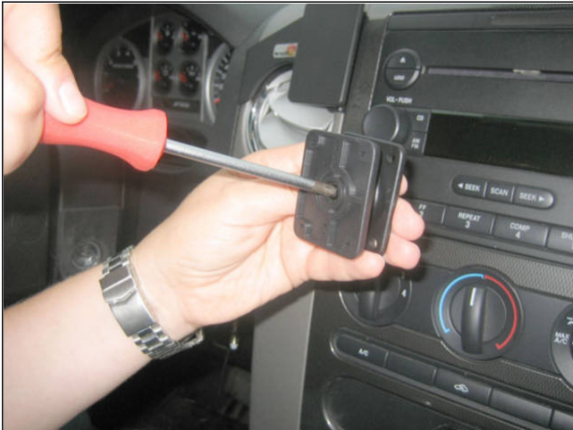
1. Unscrew the screw in the center of the holder and remove the holder from the Tilt Swivel base plate.
