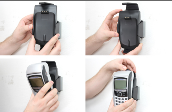
3. Place the charging unit into the holder by carefully expanding the edges of the holder while sliding the charging unit into the holder in a downward motion. To place the device in the holder: Place the bottom part of the device into the holder. Press the top of the device forward into place in the holder. To remove the device from the holder: Press the upper part of the holder forward. When the device is set free, lift it upward out of the holder.
