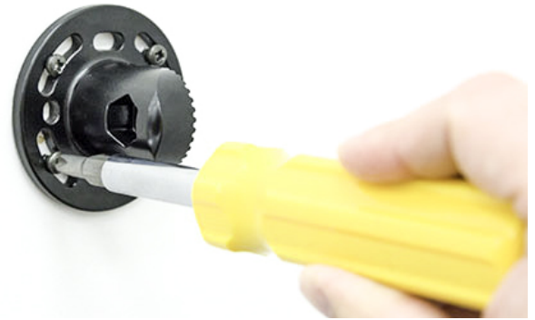
2. Fasten the pedestal base to the mounting location using the appropriate screws/hardware.
