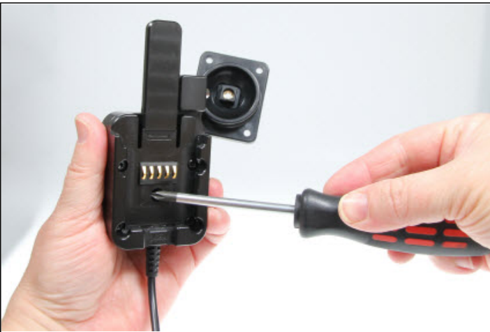
1. Unscrew the screw in the center of the power block and remove the block from the Tilt Swivel base plate.
