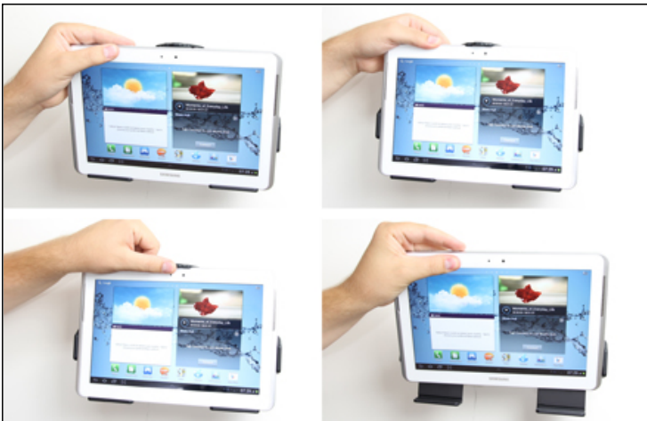
3. To place the device in the holder: Place the lower part of the device in the holder, then flip/press the upper part forwards so it snaps into place in the holder. To remove the device from the holder: Press upwards on the upper part of the holder, in the same time pull the upper part of the device out from the holder and then lift the device up and out from the holder.
