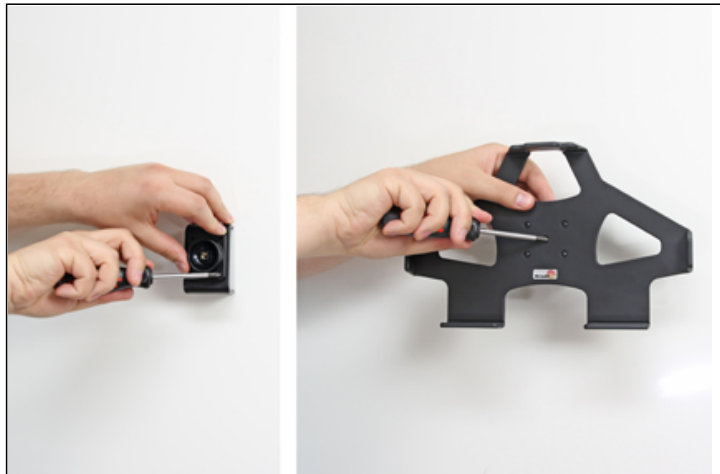
2. Place the base plate over the matching holes in your mounting bracket (demo ProClip mount shown in picture) Attach the base plate by using the self-tapping screws. Note: The machine screws with nuts are for mounts made of metal with large holes. Start to thread the center screw into the base plate. When you connect with the nut pull the holder towards you to prevent the nut from spinning around. Continue to tighten the screw firmly. Then loosen the screw slightly for easier angling/rotation of the holder.
