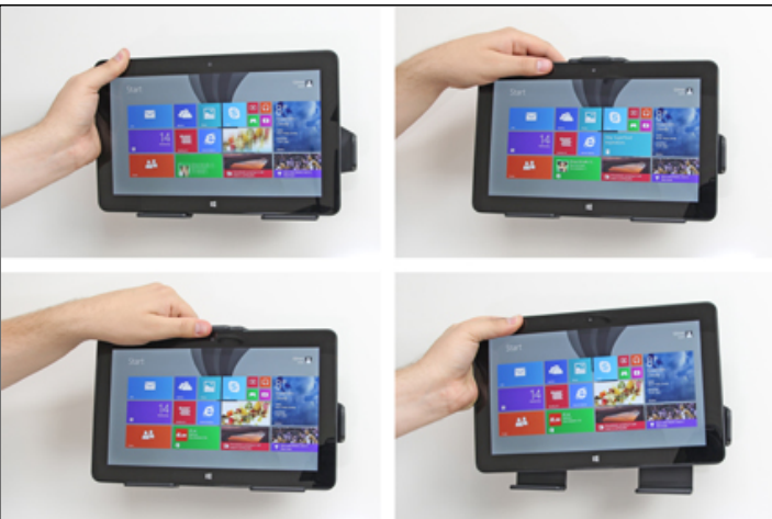
3. To place the device in the holder: Place the lower part of the device in the holder, then flip/press the upper part forwards so it snaps into place in the holder. To remove the device from the holder: Press upwards on the upper part of the holder, in the same time pull the upper part of the device out from the holder and then lift the device up and out from the holder.
