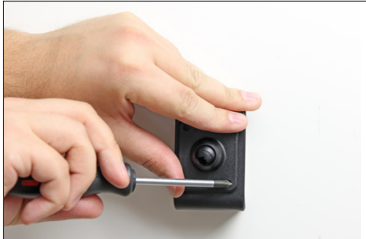
2. Place the base plate over the matching holes in your mounting bracket (demo ProClip mount shown in picture) Attach the base plate by using the self-tapping screws.
