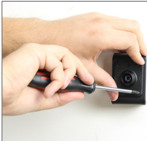
2. Place the Tilt Swivel base plate over the matching holes in your mounting bracket (demo ProClip mount shown in picture) Attach the base plate by using the self-tapping screws. Note: The machine screws with nuts are for mounts made of metal with large holes.
