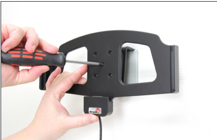
3. Place the holder onto the tilt swivel base plate and reattach it with the center screw. The center screw also controls the pivot, tighter for a firm hold and loose for easier rotation/angling of the Holder.
