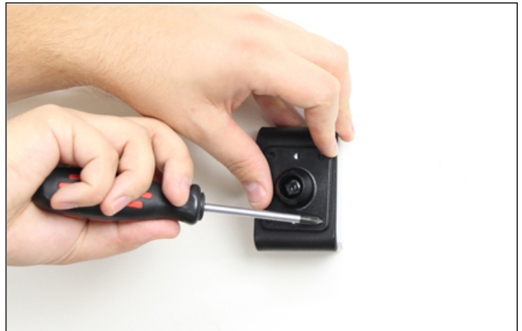
2. Place the base plate over the matching holes in your mounting bracket (demo ProClip mount shown in picture) Attach the base plate by using the self-tapping screws. Note: The machine screws with nuts are for mounts made of metal with large holes.
