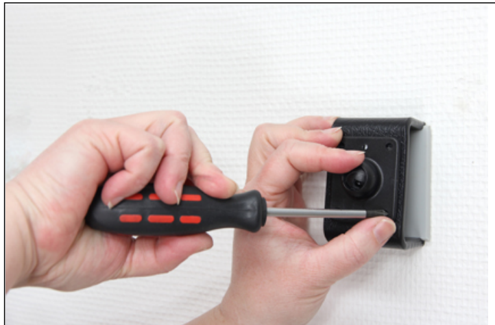
2. Place the Tilt Swivel base plate over the matching holes in your mounting bracket (demo ProClip mount shown in picture) Attach the base plate by using the self-tapping screws. Note: The machine screws with nuts are for mounts made of metal with large holes.
