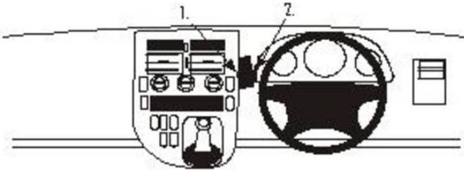
1. Clean the surface at pos. 1 with the enclosed alcohol pad. Peel off both adhesive tape covers on the ProClip.
