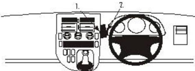
3. Press the right part of the ProClip, with adhesive tape, into the gap at pos. 2.
