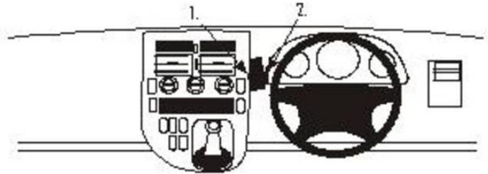
2. Press the left part of the ProClip, with curve, into the gap at pos. 1.
