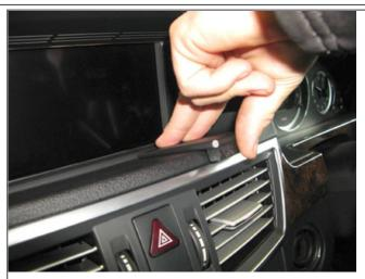
2. Press down on Part 1 so the adhesive tape attaches.
