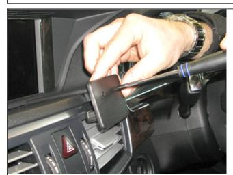
3. Open up the predrilled holes in Part 2 with a screwdriver. Peel off the adhesive tape cover on Part 2. Place Part 2 onto Part 1 so the holes match. Attach Part 2 onto Part 1 with the enclosed screws.
