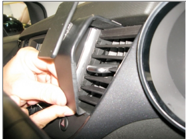
2. Press the lower part of the ProClip upward and forward. Hook the angled edge on the lower part of the ProClip into the gap between the air vent and the center console.
