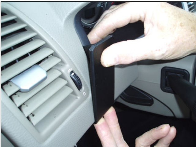
3. Press forwards on the upper part of the ProClip so the grooved edge goes into the gap between the frame surrounding the instrument panel and the dashboard. Press until you hear/feel it snaps into place
