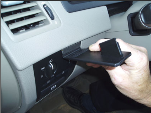
1. Peel off the over of the adhesive tape on the ProClip. Press the angled edge on the lower part of the ProClip into the gap in the dashboard.
