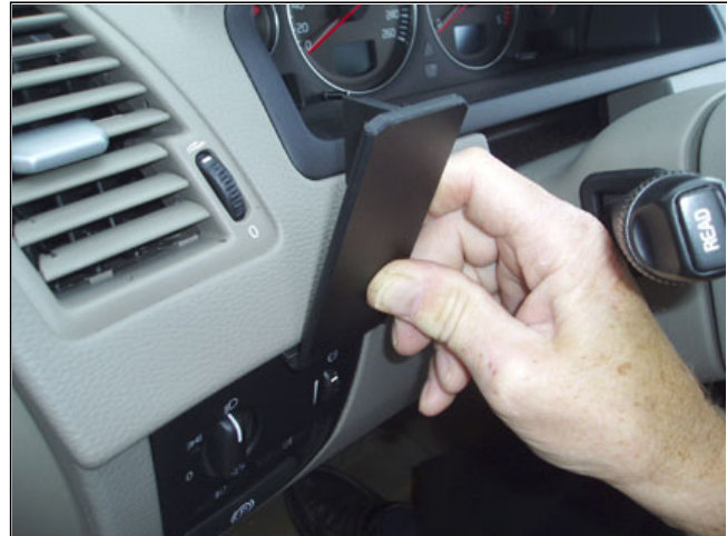
2. Press the ProClip upwards/forwards so the angled lower edge hooks into the gap.
