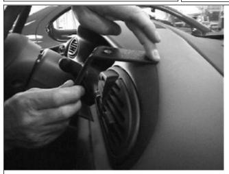
1. Peel off the cover of the adhesive tape on the ProClip. Press/hook the angled edge on the upper part of the ProClip into the gap between the panel frame and the padded dashboard.
