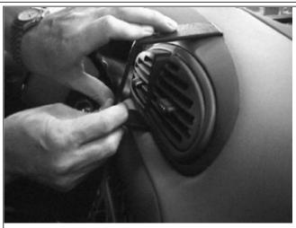
2. Press the grooved edge on the lower part of the ProClip into the gap between the air vent panel frame and the padded part of the dashboard. Press until you see or hear/feel it snaps into place.
