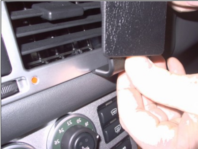
1. Press the lower part of the ProClip into the gap between the the dashboard and the frame surrounding the air vent.
