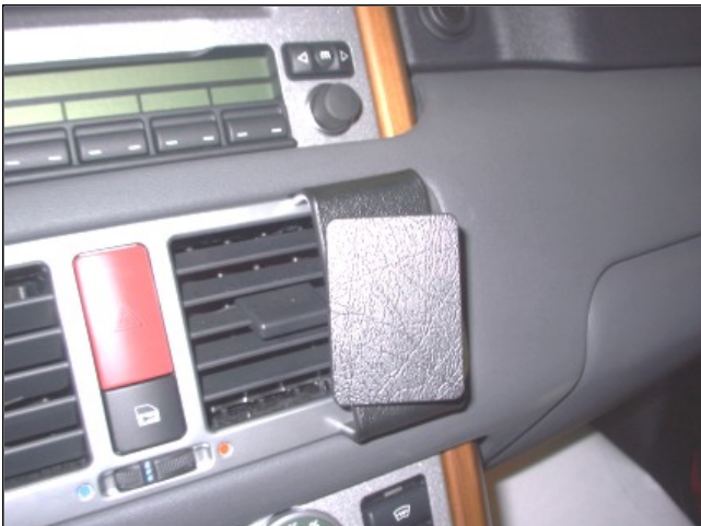
3. The ProClip is now in place as shown here and in the overview picture.
