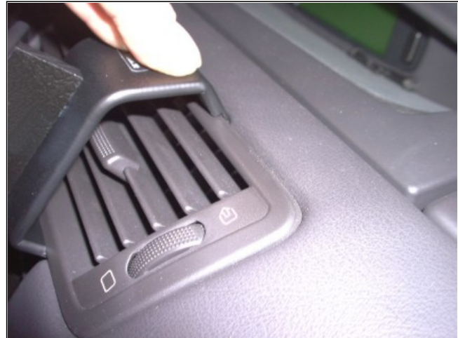
2. Press forwards on the ProClip so the upper part snaps into the gap between the frame surrounding the air vent and the dashboard.
