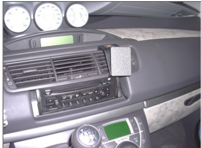
4. The ProClip Mount is in place.
