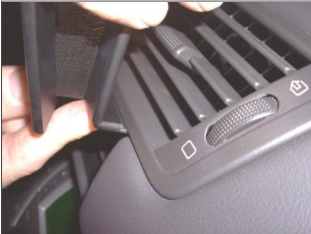
1. Hook the lower part of the ProClip under the frame surrounding the air vent.
