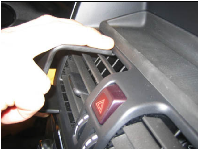
3. Press the upper part of the ProClip downward and then forward. Release the pressure when the grooved upper edge is in the air vent so it hooks into the upper edge of the air vent.
