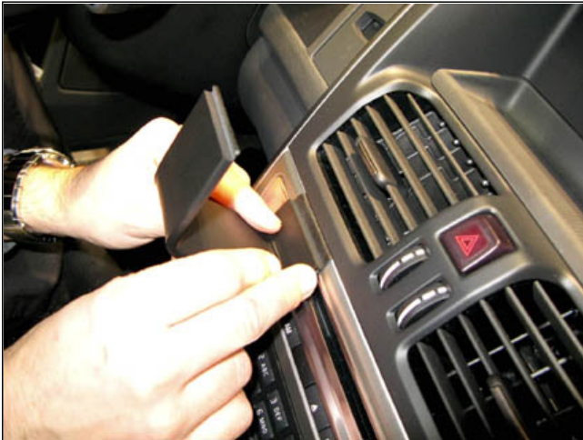
1. Press the curved edge on the lower part of the ProClip into the gap between the frame surrounding the air vent and the control panel.
