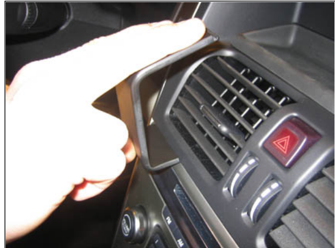
2. Flip the upper part of the ProClip upward/forward so the curved edge hooks behind the control panel.
