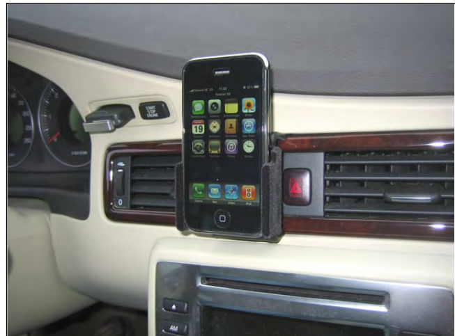
4. Slide the device down into the holder.
